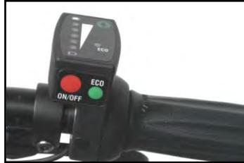
The twist grip incorporates a display and operating unit with a number of pushbuttons and light-emitting diodes (LEDs).
