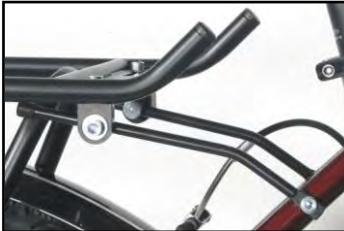
Mount the luggage carrier so that the luggage carrying area is horizontal. Make sure that sufficient clearance is left between the luggage carrier and the mudguard to allow subsequent mounting of the control unit at the end of the luggage carrier.
