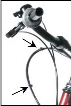
Tie the twist grip cable and the brake and gear cables together with cable ties or coiled cable. Make sure that the cables do not restrict handlebar lock-to-lock movement.
