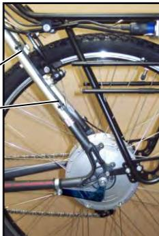
Introduce the front wheel with the spoked-in motor into the front fork or the rear wheel into the rear triangle.
