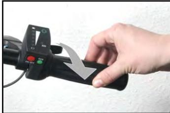
Remove the handlebar grips.
