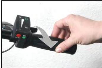
The system must be switched off to start with! To check the automatic return, twist the twist grip backwards and then release (see photo). The twist grip must immediately return to its initial (zero) position.
