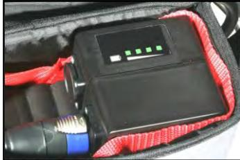
All batteries usually leave the factory fully charged. However because there is always a certain amount of self-discharge (typically ~1% per day at room temperature) the battery should be charged up before being used for the first time.
