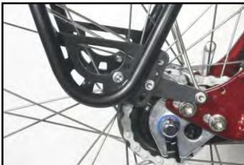
Now attach the bottom of the luggage carrier with two socket head screws (Allen screws) and self-locking nuts to the dropout ends of the rear triangle on both sides, using the extension plates.
