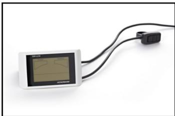
The control unit can be mounted either on the left side or the right side or even in the middle of the handlebar. The control elements (e.g. gears) may have to be mounted on the opposite side. The fixing clamp is available for handlebar diameter Ø22 mm or Ø31,8 mm optionally.
